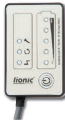
Figure 2: External state of charge and status display
